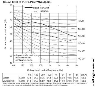
•Depending on the operation conditions, the unit generates noise caused by valve actuation, refrigerant flow, and pressure changes when operating normally. Please consider to avoid location where quietness is required. For BC controller, it is recommended to be installed in places such as ceilings of corridor, rest rooms and plant rooms.
