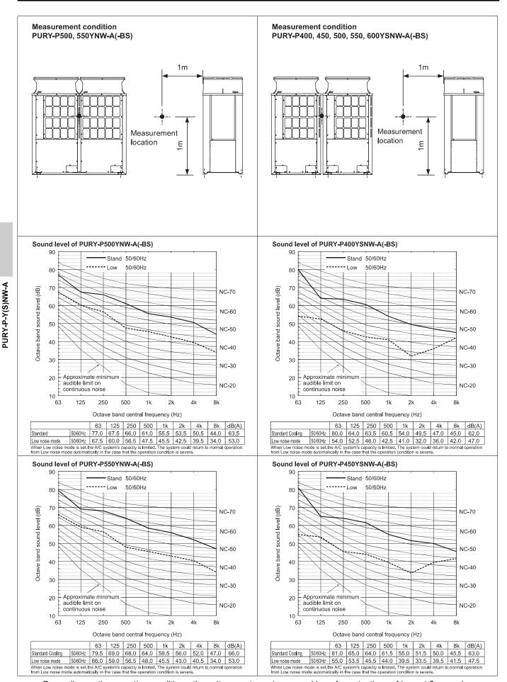
•Depending on the operation conditions, the unit generates noise caused by valve actuation, refrigerant flow, and pressure changes when operating normally. Please consider to avoid location where quietness is required. For BC controller, it is recommended to be installed in places such as ceilings of corridor, rest rooms and plant rooms.
