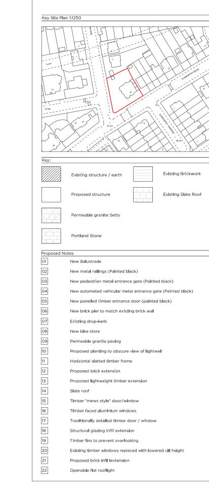
31.07.2019 Issued For Planning 1. Height of parapet reduced by 200mm 2. Extension centred between chimney breasts 3. Depth of reveal reduced
