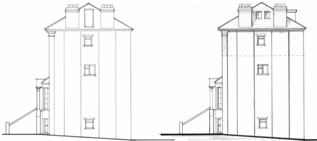
Figure 13: (left) existing side elevation arrangement showing set back cut-away roof access hatch door; (right) 2018 arrangement approved at appeal for the introduction of two new conservation roof lights. Source: Allen Smith Associates.
