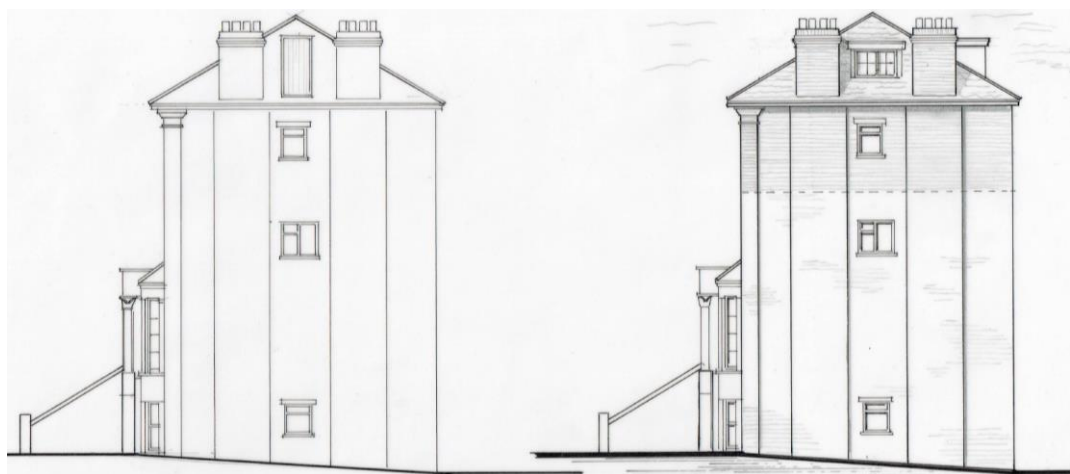
Figure 14: (left) existing side elevation arrangement showing set back cut-away roof access hatch door; (right) arrangement of side elevation proposed by this appeal, which seeks to introduce a single dormer window in place of the conservation roof lights. Source: Allen Smith Associates.
