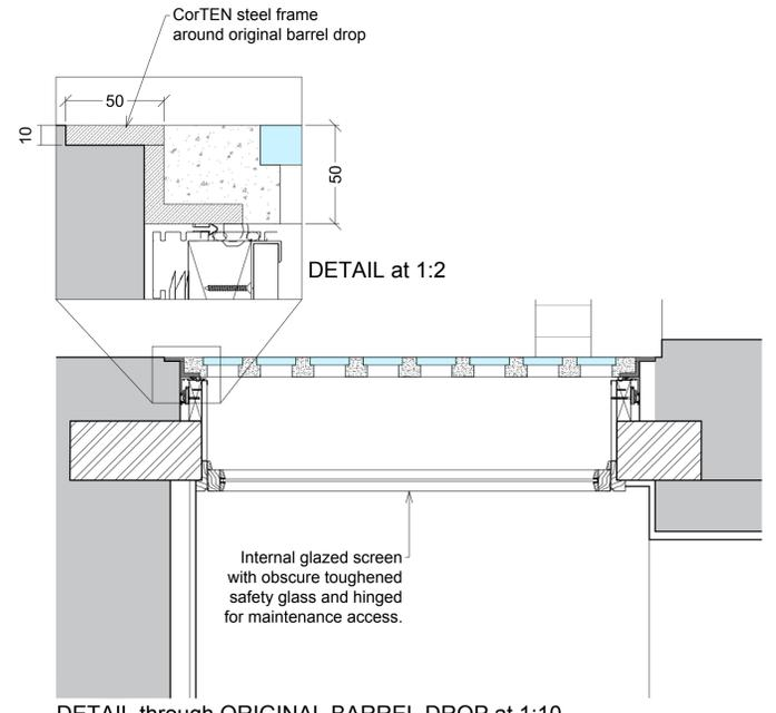
Rev. B, 25th Sept 2019: 50mm wide CorTEn steel frame shown around original barrel drop
