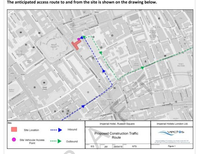
Construction routing will utilise the existing highways network to and from Queen Square, via the A40 and A401. Queen Square currently accommodates large vehicles and access is provided on a one-way loop arrangement via Old Gloucester Street and Boswell Street.
