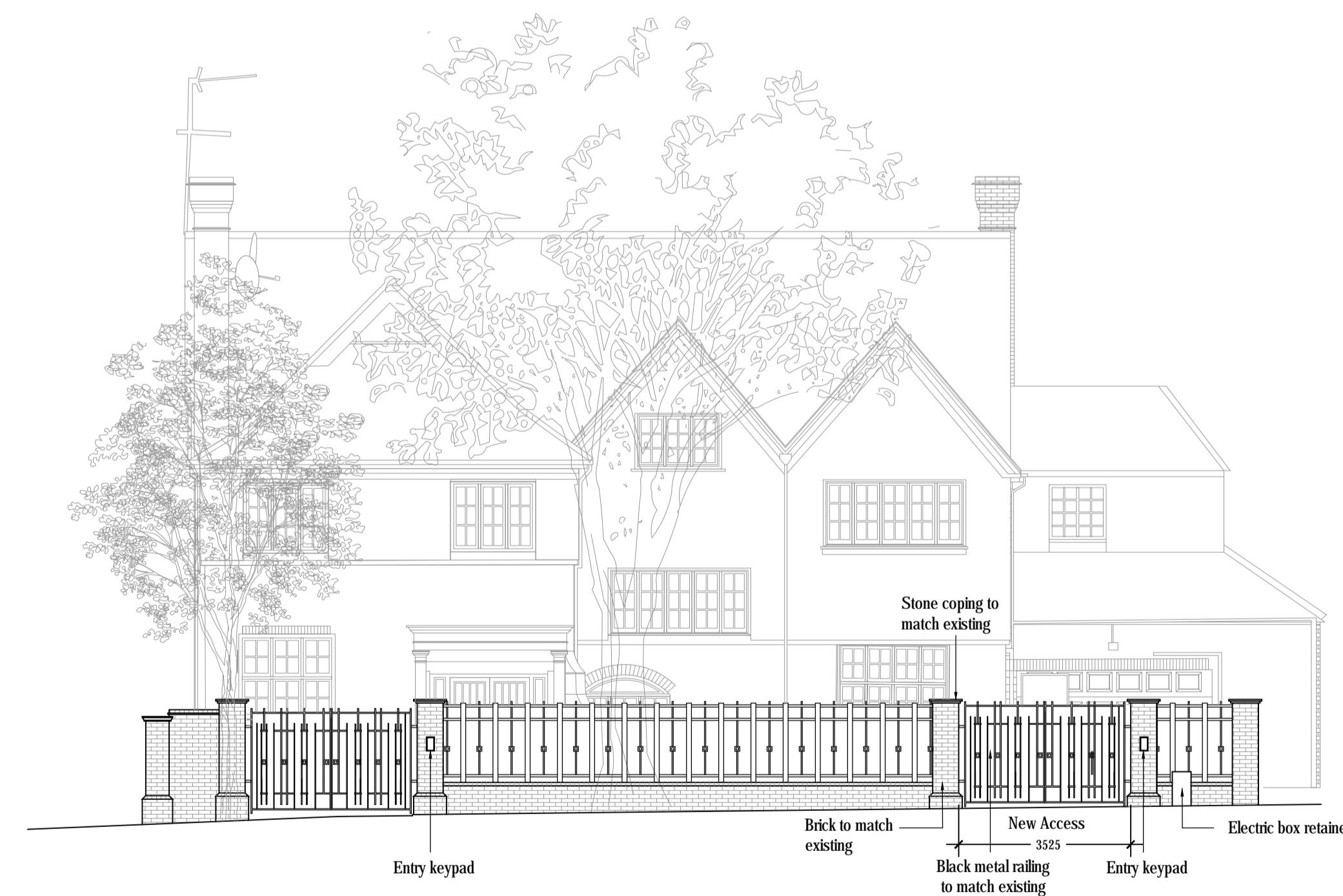
Proposed Front Elevation SCALE 1:100@A1
