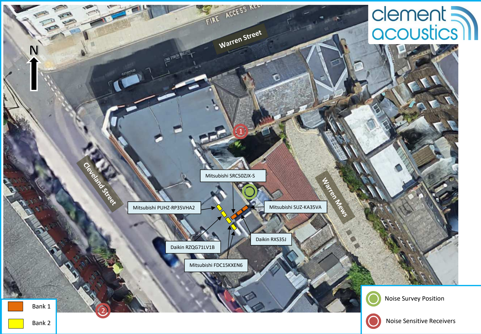
15055-SP1 Indicative site plan indicating noise monitoring position and nearest noise sensitive receiver.
