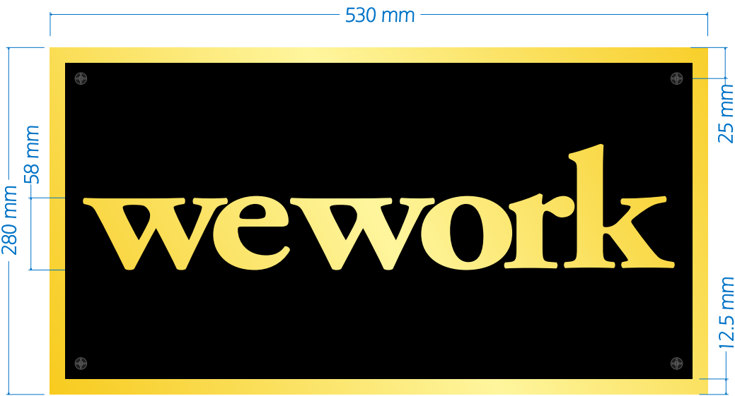
Sign P4 - 1 no. 3mm brushed brass plaque with raised text and border, acid etched and in-filled in black.
