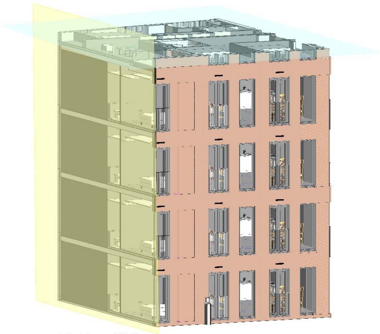
3D study of the façade for Flat type A6.08.02 illustrating MVHR intake and extract ventilation grilles
