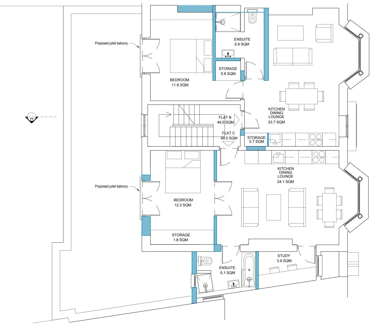
All drawings to be read in conjunction with structural engineer's and service engir Blue linework shows proposed wall
