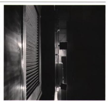
For further comparison, a bank of conventional "Z" section louvre was also put on trial. For extra rain resistance, the louvre incorporated a front edge rain channel and a wire mesh between each blade,
