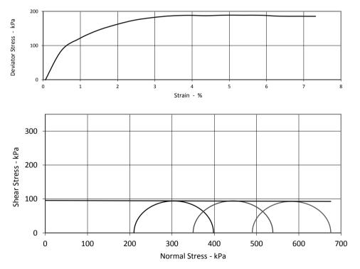
Unconsolidated Undrained Shear Strength Tested in Accordance with BS 1377: Part 7: 1990
