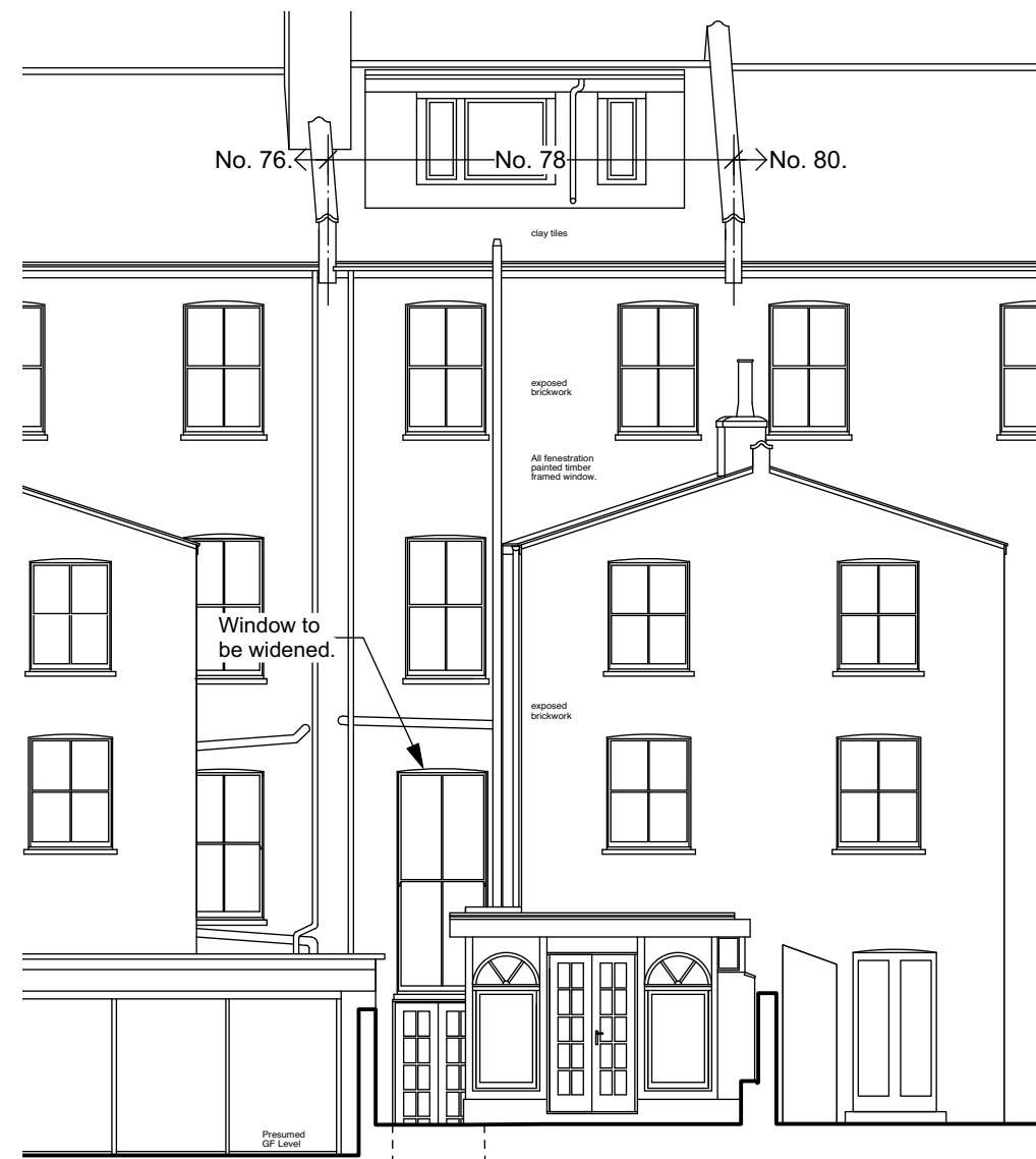
EXISTING REAR ELEVATION
