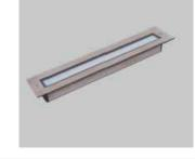
REF 'A1' LUMINAIRE CEILING RECESSED LED DOWNLIGHT. 7.6 W, 500lm-3000lm, 2700K-4000K, CR180+. 80mm (W) x 81mm (D) OPTIONAL: 3HR MAINTAINED EMERGENCY BACK UP, DIMMING CONTROL, DALI. LOCATION: CIRCULATION
