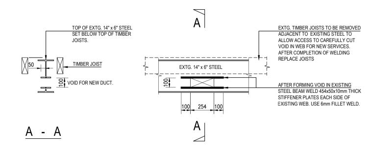
FORMATION OF SERVICE VOID IN EXISTING STEEL FLOOR BEAM
