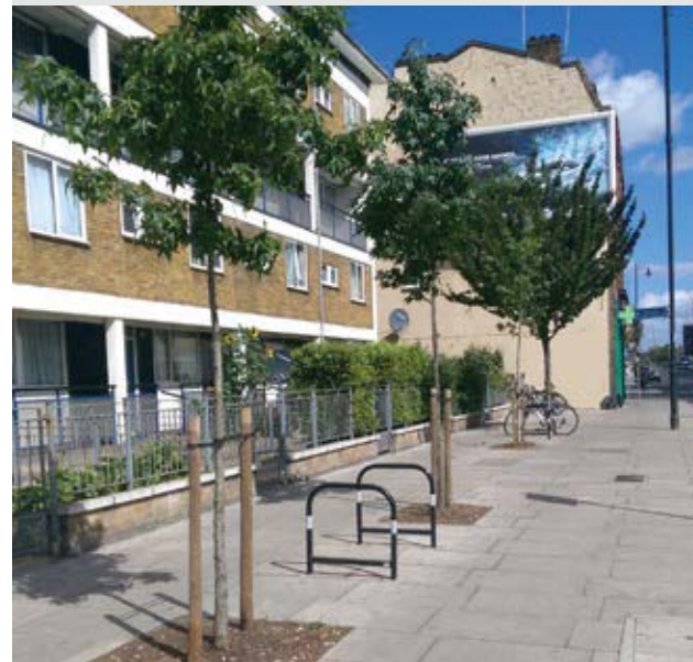
Figure 200: A street furniture zone of cycle parking and trees located at the back of the footway
