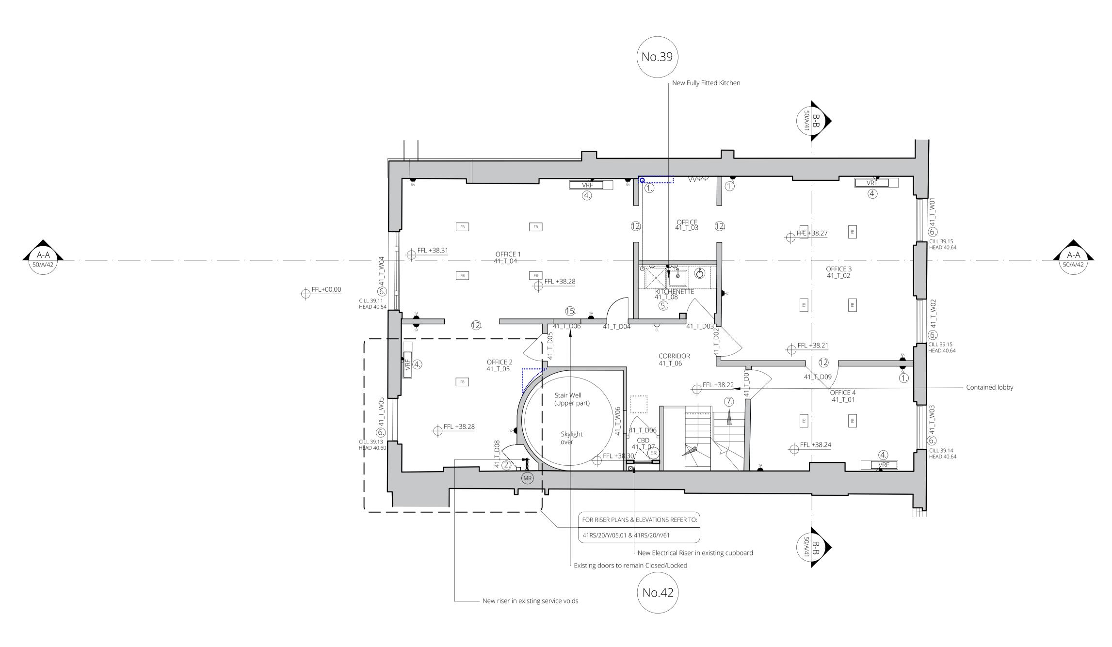
Note: Electrical DB for Third Floor to be located in Second Floor.
