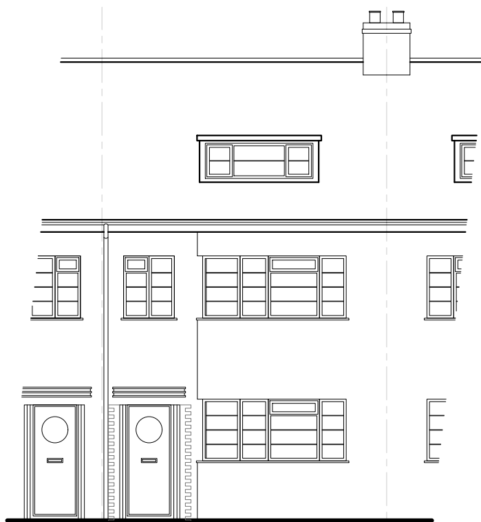
Front Elevation As Existing - Scale 1:100
