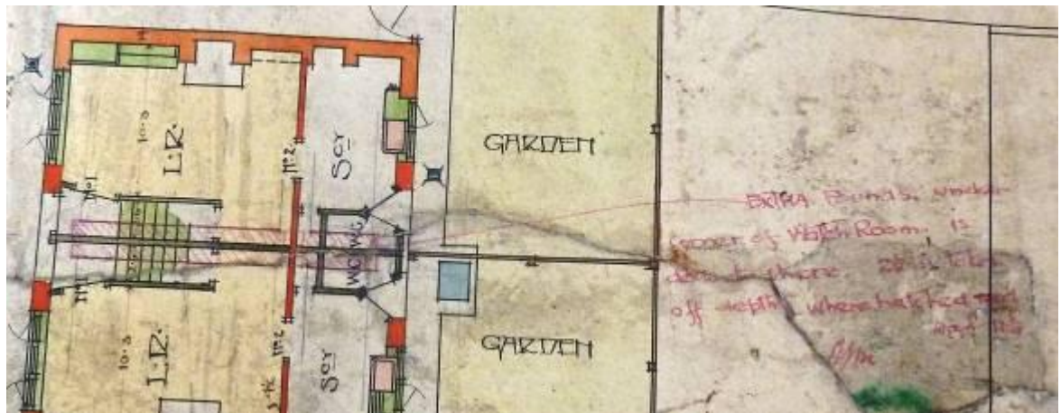
Fig 9.1.7: Highlighted note of reduced foundation concrete to dividing wall
