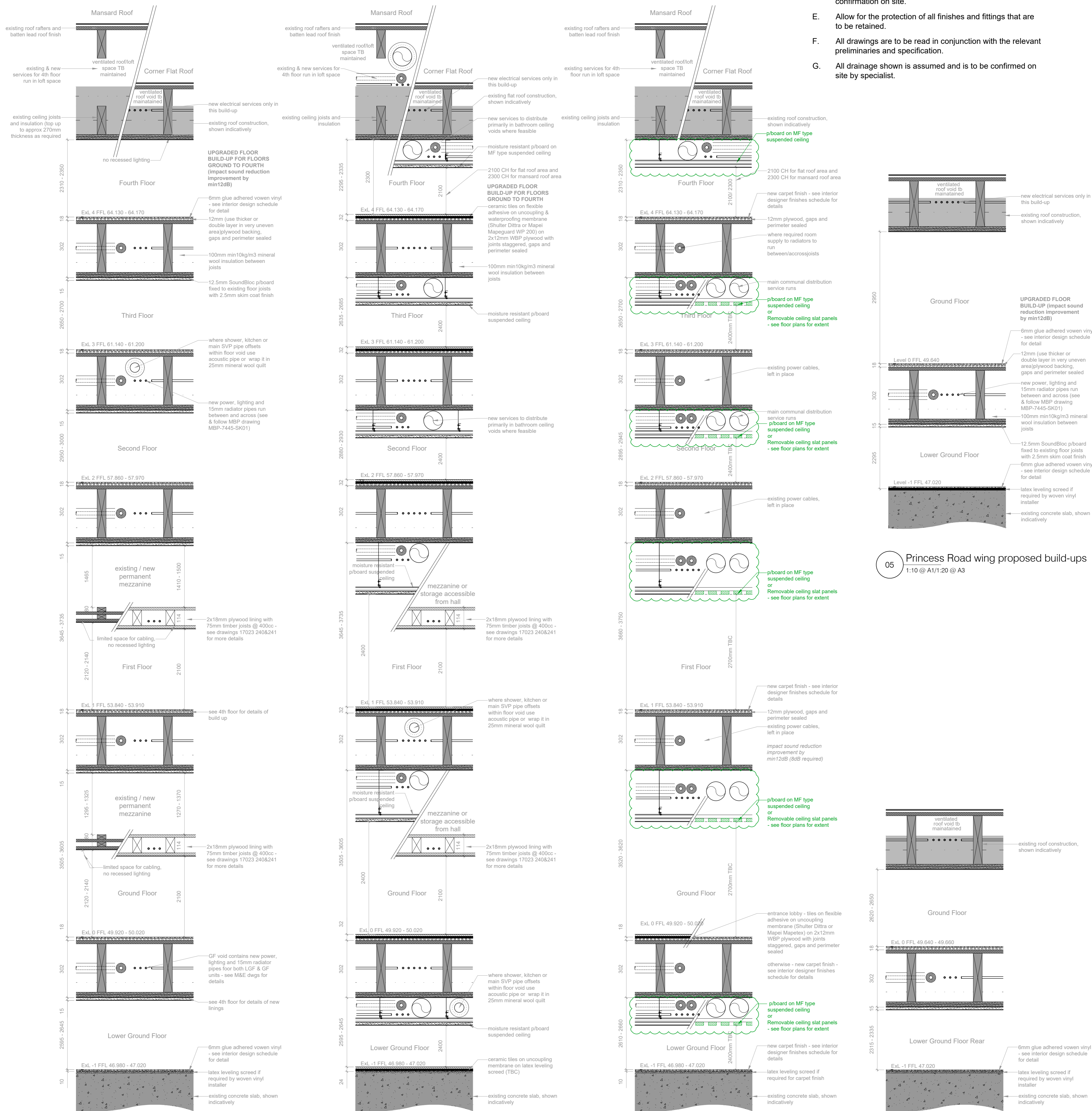
01 Main building proposed floor build-ups 1:10 @ A1/1:20 @ A3
