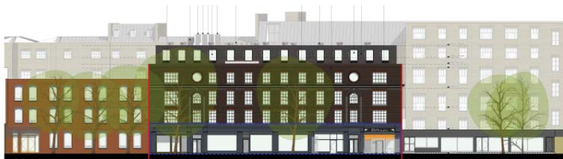
Consented Front Elevation showing roof extension at 175-185 Gray's Inn Road prepared by Bond Bryan Architects
