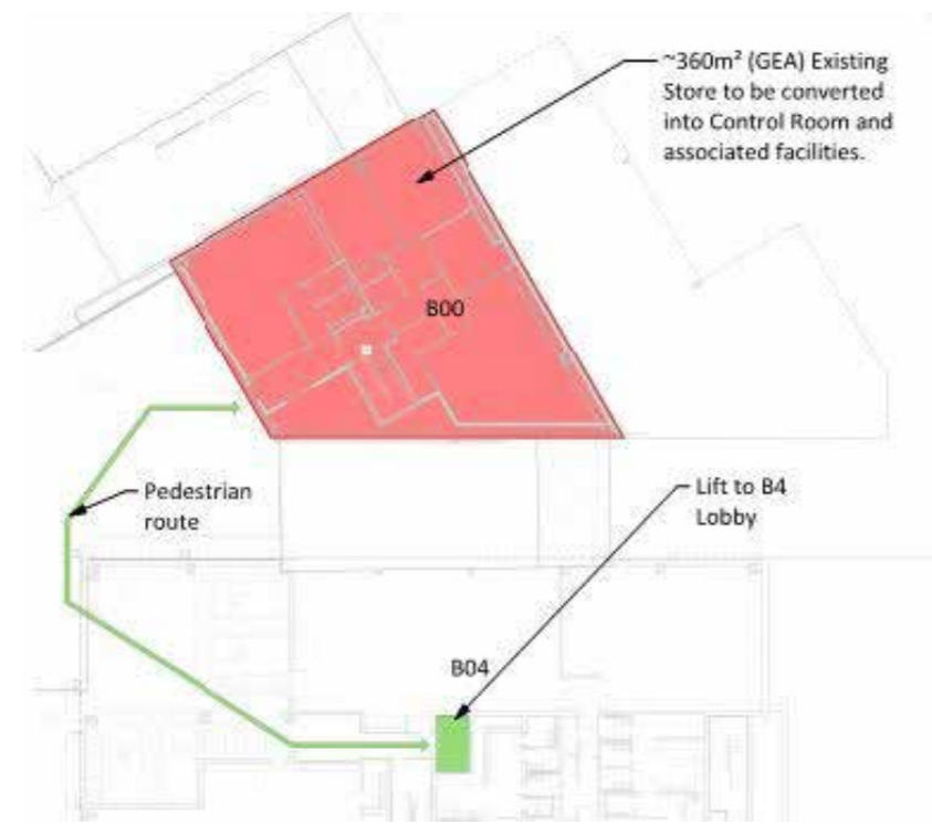
Figure 15: Access routes and lift location for level -03
