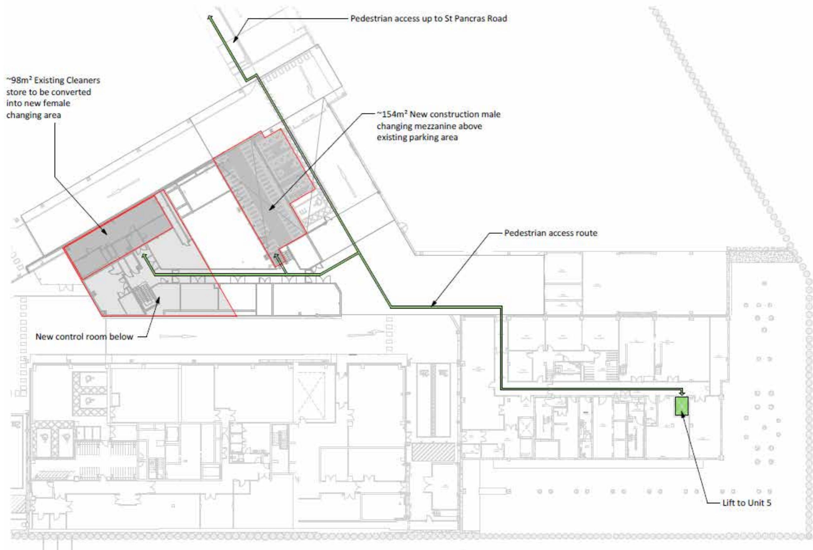
Figure 4: Proposed internal pedestrian route from Unit 5 (Building B6) to the shared Zone B basement
