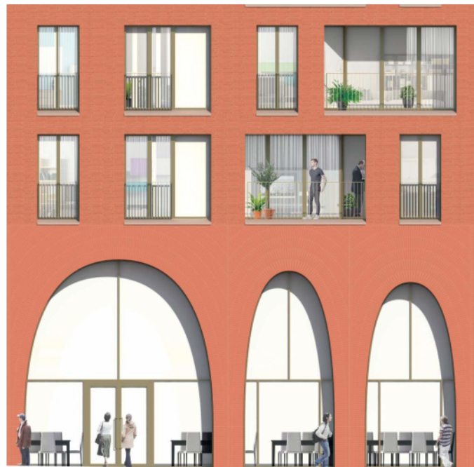
Figure 4: Typical arch brick arrangement showing the "Coursing Rings" bond and the updated all red brick blend
