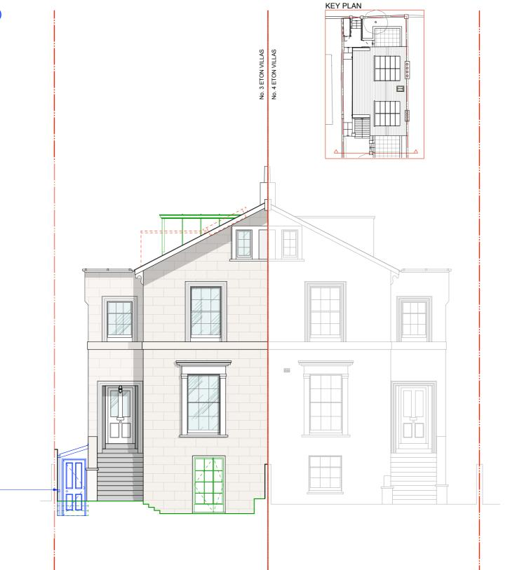
NEW SIDE PASSAGE LEAN-TO WITH GLAZED ROOF SET INTO LIGHTWEIGHT TIMBER STRUCTURE TO SHELTER PASSAGEWAY WITH TRADITIONAL TIMBER DOORS AT BOTH ENDS
