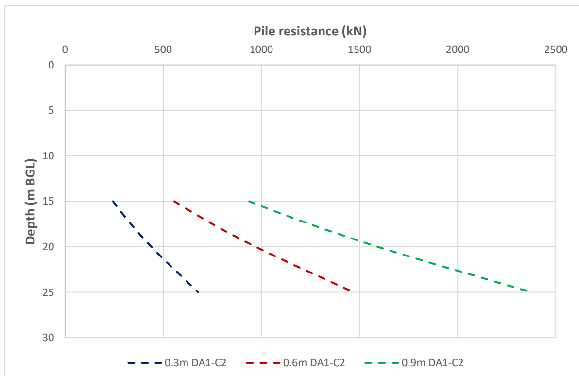
Figure 7-A: Graph showing variation of pile resistances with toe level for Combination 2 for a selection of pile diameters
