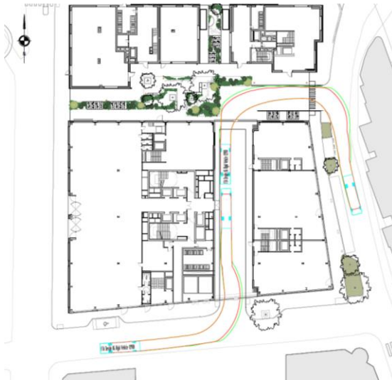
Figure 3.6 Refuse (7.9m) servicing street tracking
