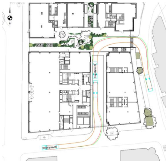
Figure 3.7 HGV (10m) servicing street tracking
