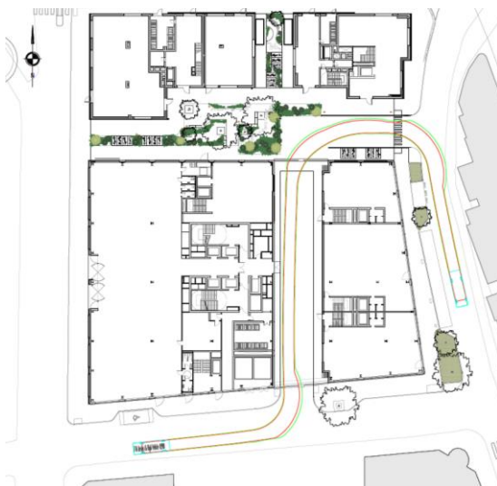
Figure 3.5 LGV (7m) servicing street tracking
