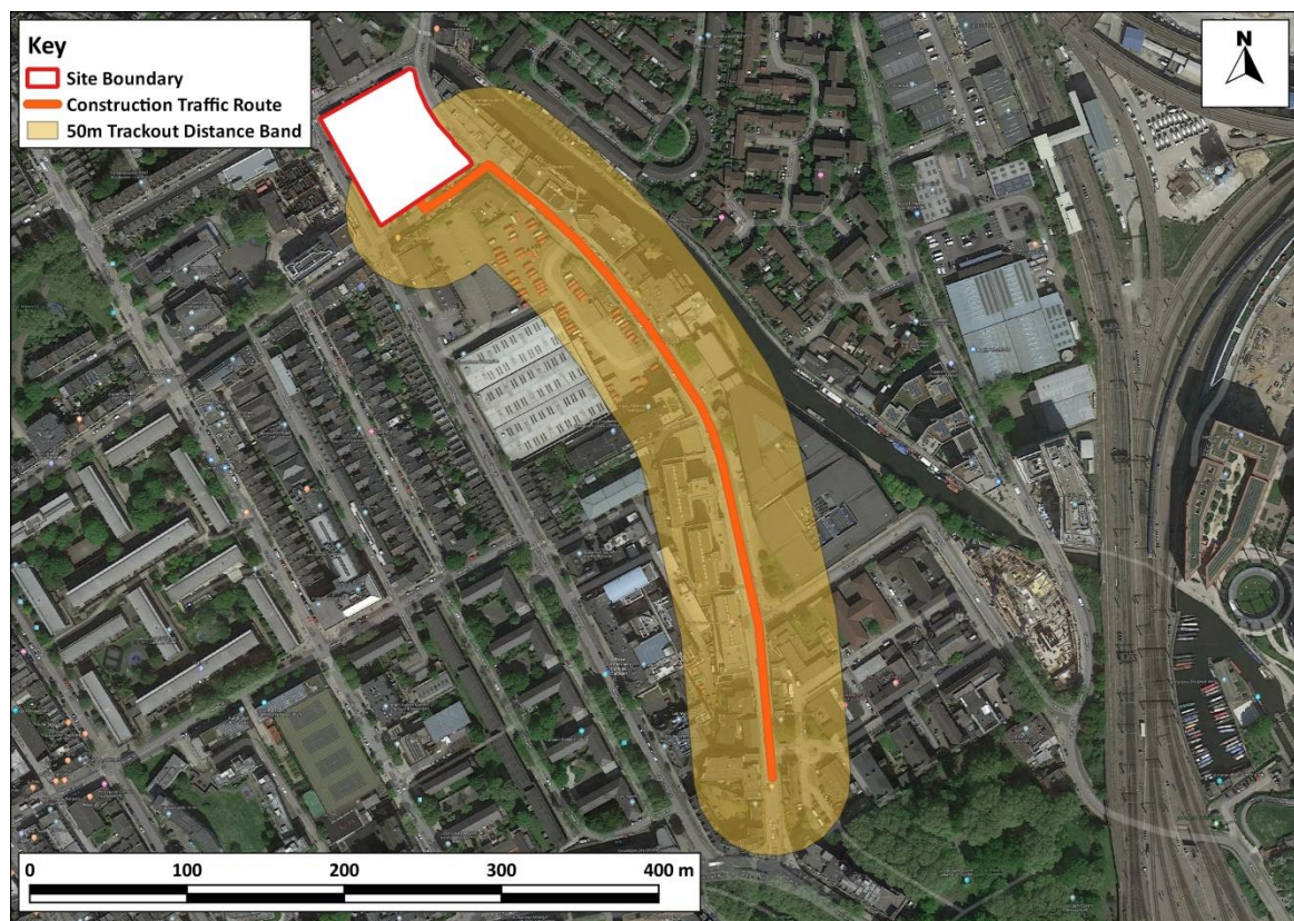
Figure 4: 50 m Distance Band around Roads Used by Construction Traffic Within 500 m of the Site Exit
