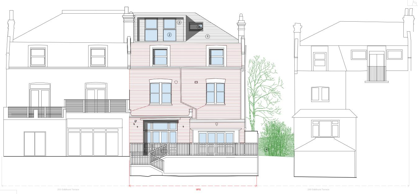
New glazing - Timber frame windows to match existing at front, and aluminium frame to rear.
