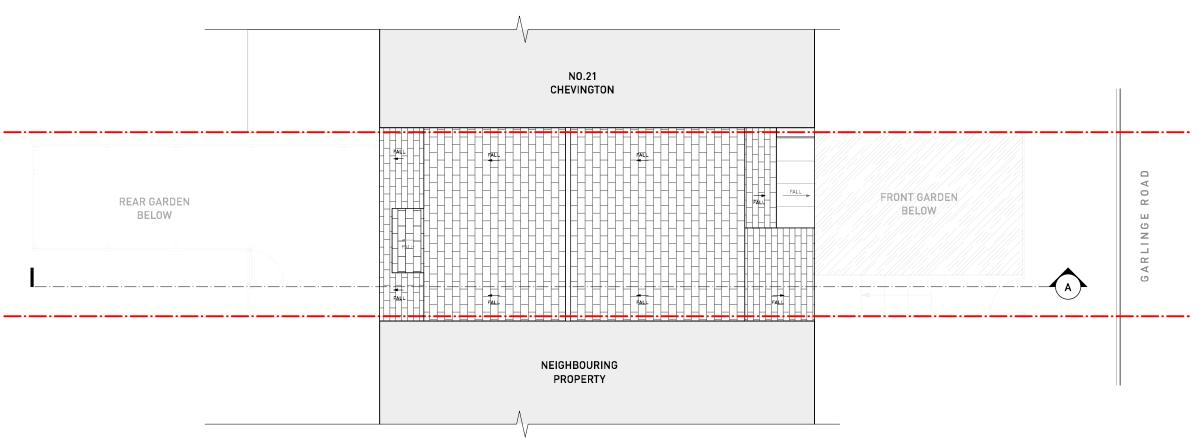
1 Existing Roof Plan Scale: 1:100
