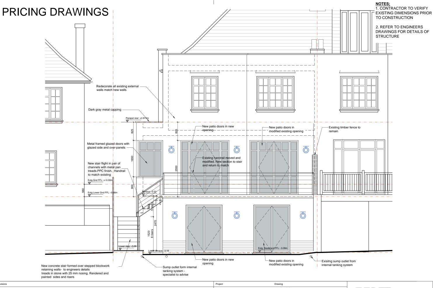
Revisions **PROPOSED** 14 Makepeace Avenue A 20.03.19 Note regarding colour of metal frames removed B 26.03.19 Existing handrail removed Holly Lodge Estate **REAR ELEVATION** C 02.08.19 Coordinated with engineers drawings and details added Revision Drawing No 1. This drawing and all the designs herein are the sole property of HAT and may not be used without written authorisation.
