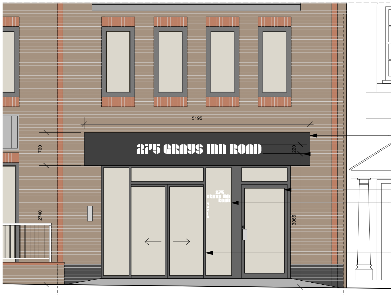
1 PROPOSED ENTRANCE ELEVATION Scale: 1:25 @ A1/1:50 @ A3
