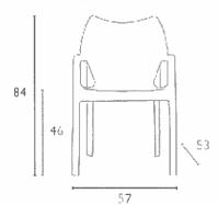
**Technical Specification** Injection of polypropylene reinforced with glass fibre
