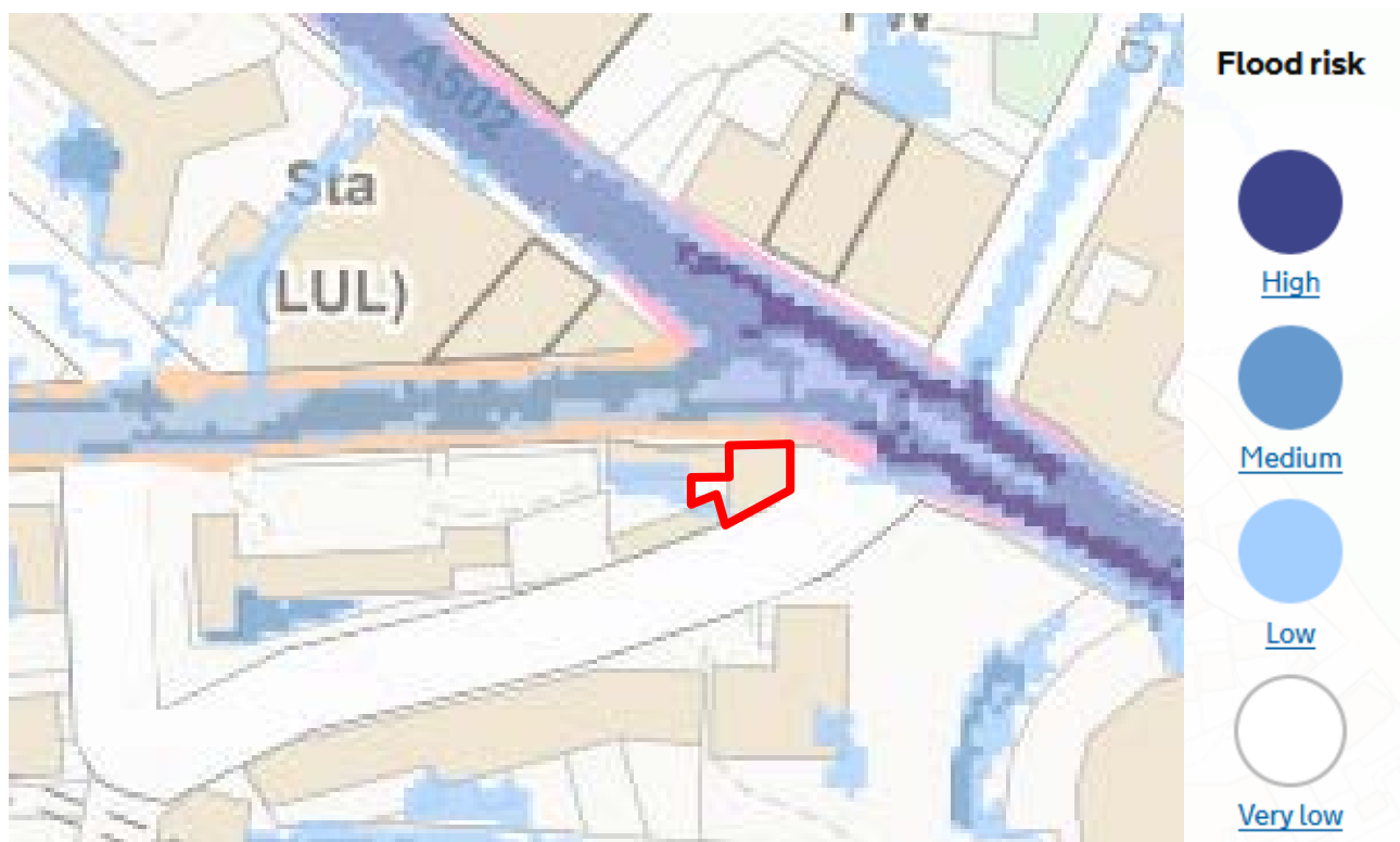
Extract of the EA's Surface Water Flooding map showing the flood risk from surface water
