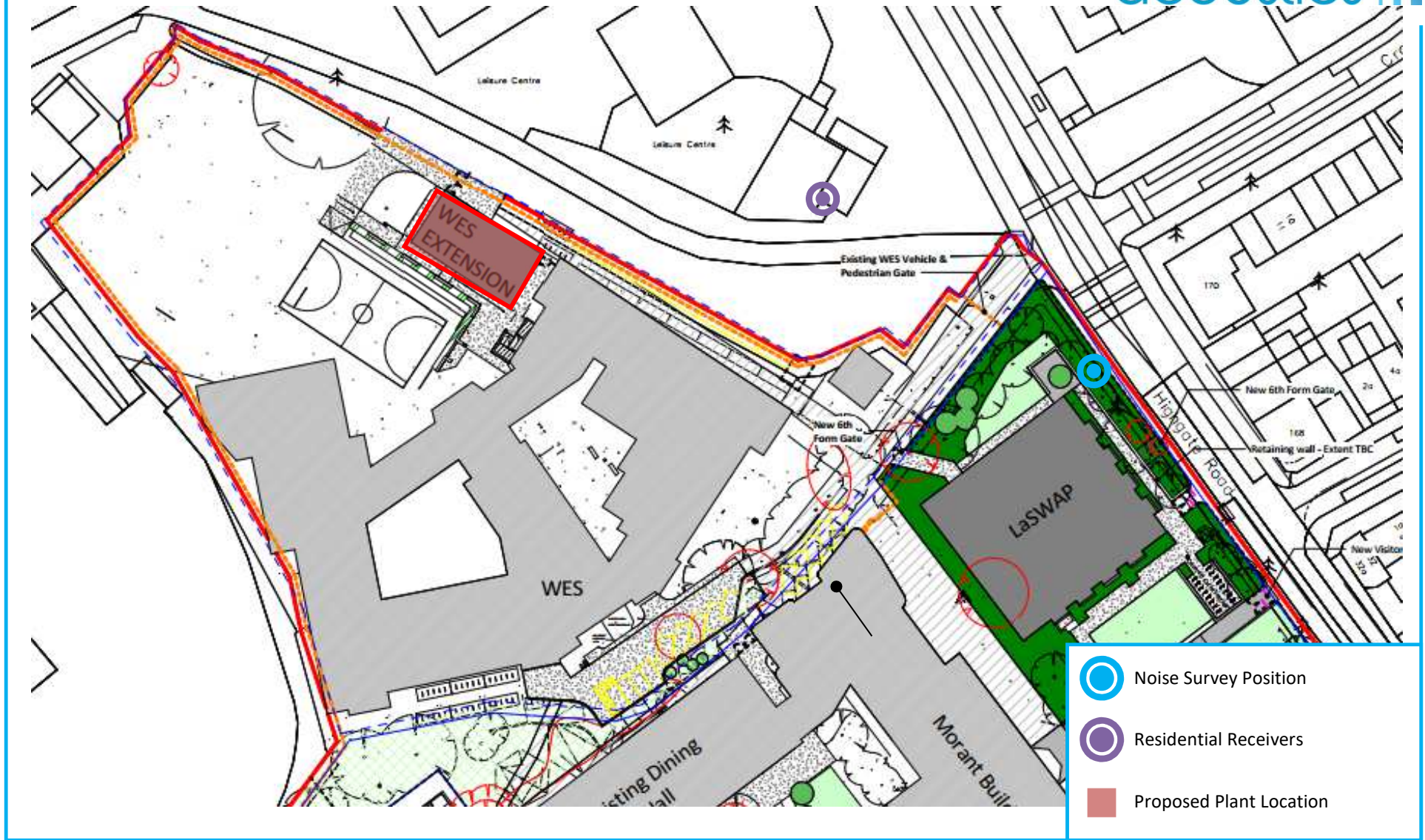
10883-SP2 Indicative site plan indicating noise monitoring position and nearest noise sensitive receivers
