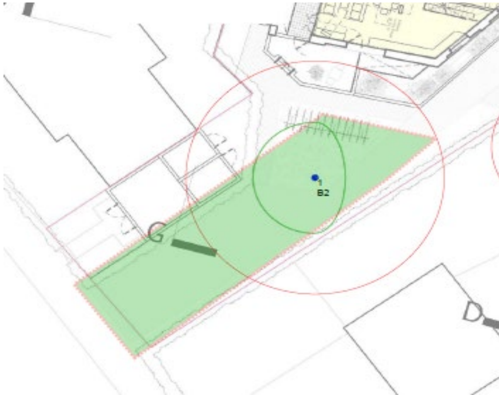
Figure 3: Extract from 2016 Arboricultural Implications Report showing extent of proposed access and location of T1.
