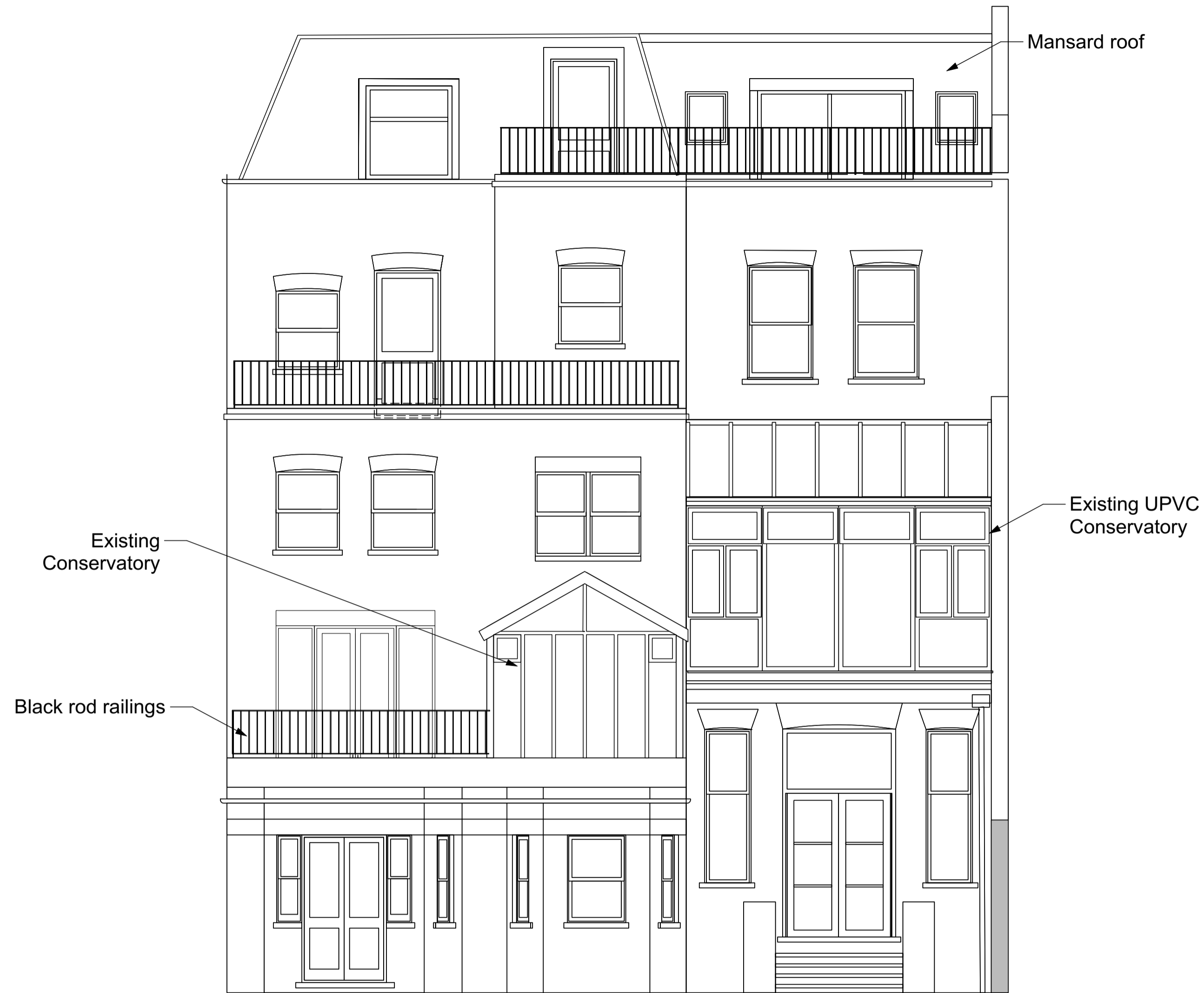
1 Existing Rear Elevation
