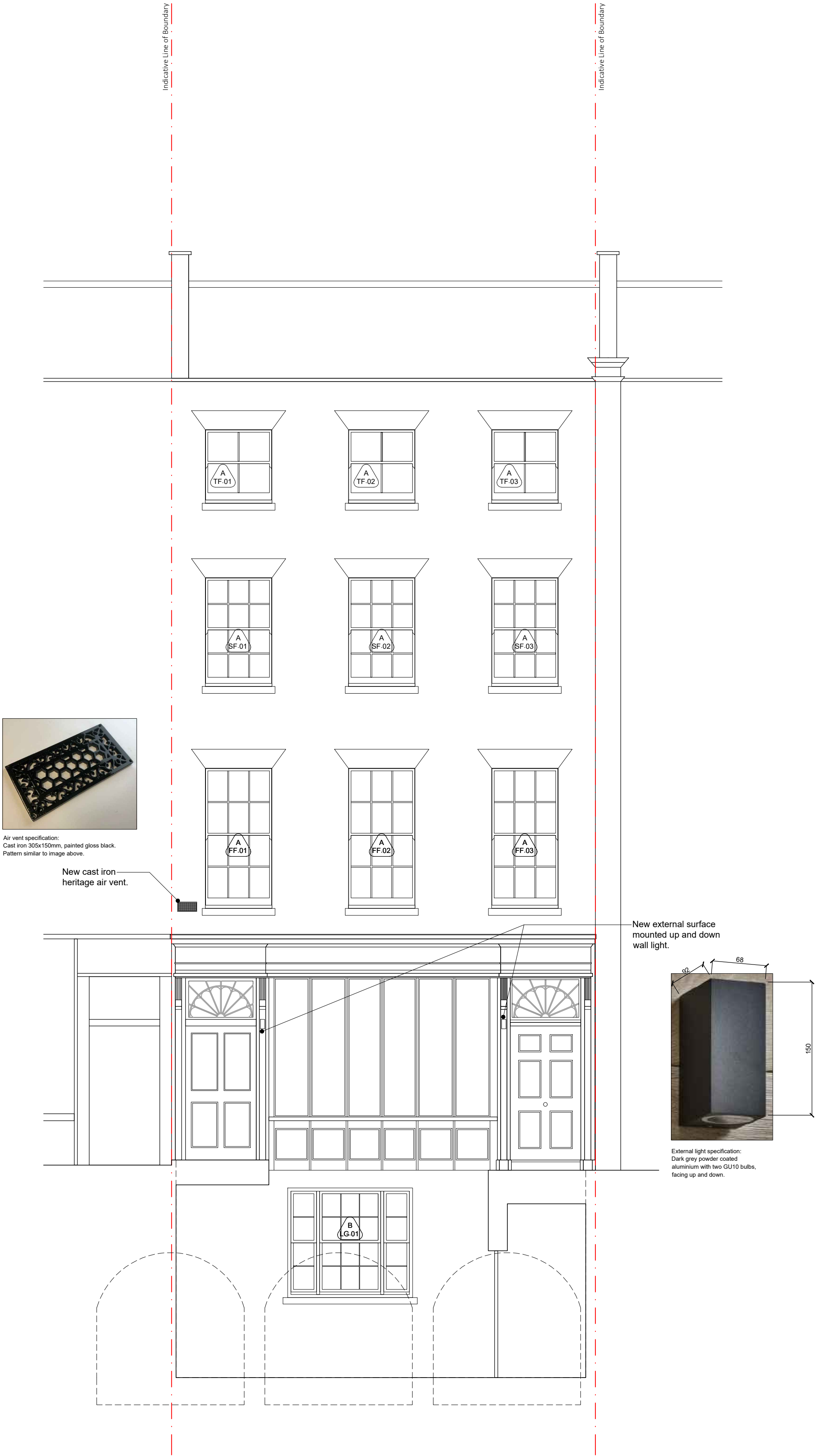
Architectural drawing showing the proposed street elevation and section CC. The elevation features a symmetrical facade with two main doorways, each topped with a pediment and a transom, and a central window wall. The section below, labeled "Section_CC", shows three arched openings. The first arch is labeled "Dressing Room" and the second is labeled "Bathroom". Dashed lines indicate the vertical alignment between the section and the elevation. Proposed Street Elevation Section_CC
