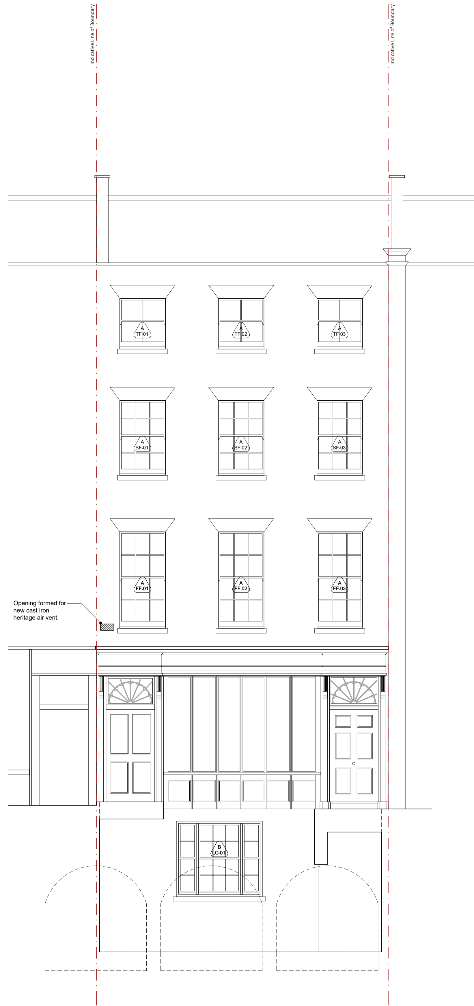
Proposed West Elevation Section_BB
