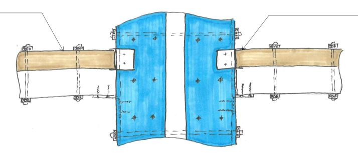
New timber joists to be supported on new joist hangers fixed to top of steel angles with 2no. 5.5mm dia. self drilling self tapping screws
