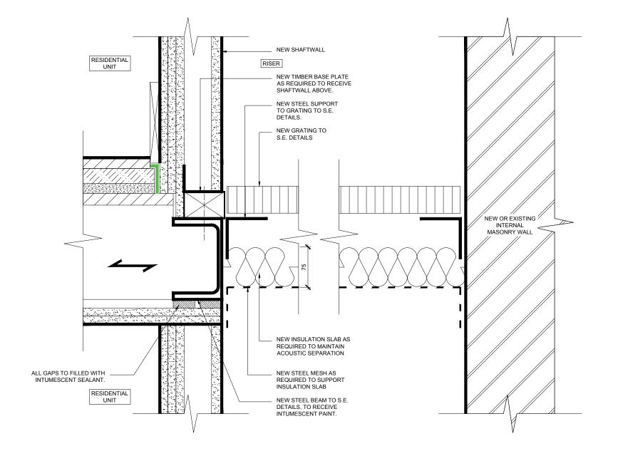
PROPOSED ACOUSTIC SEPARATION WITHIN RISER - SECTION DETAILS
