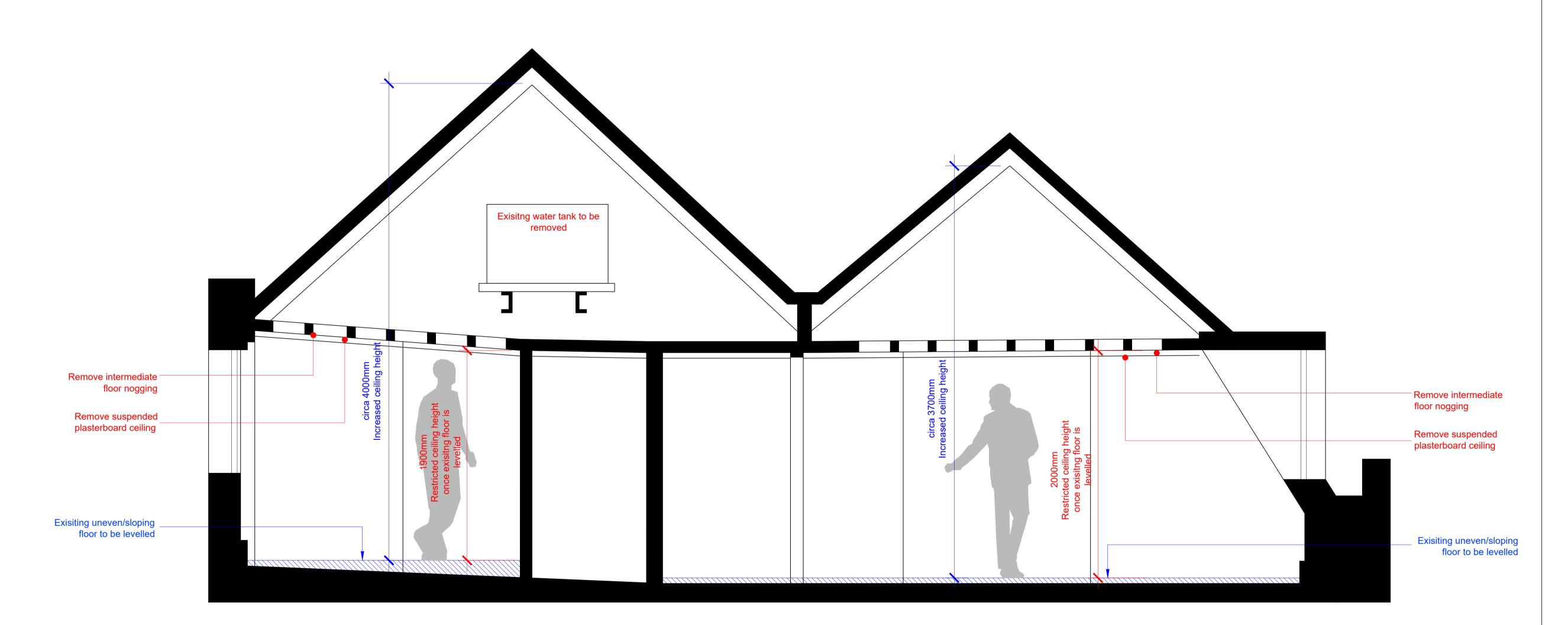
01 Existing & Proposed Internal Elevation/Section CC at No.16 - Level 3
