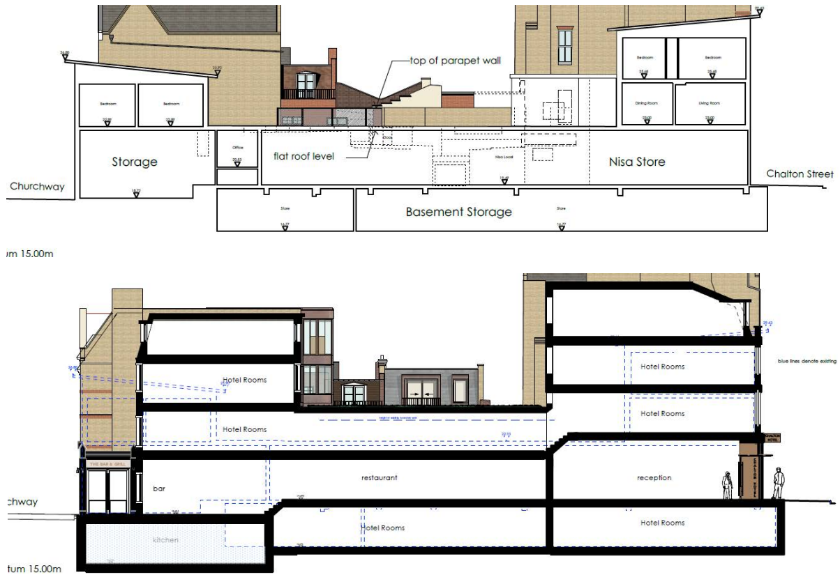
Figure 1.3 Cross section A-A' through 53-55 Chalton Street and 60 Churchway (existing above, proposed below)
