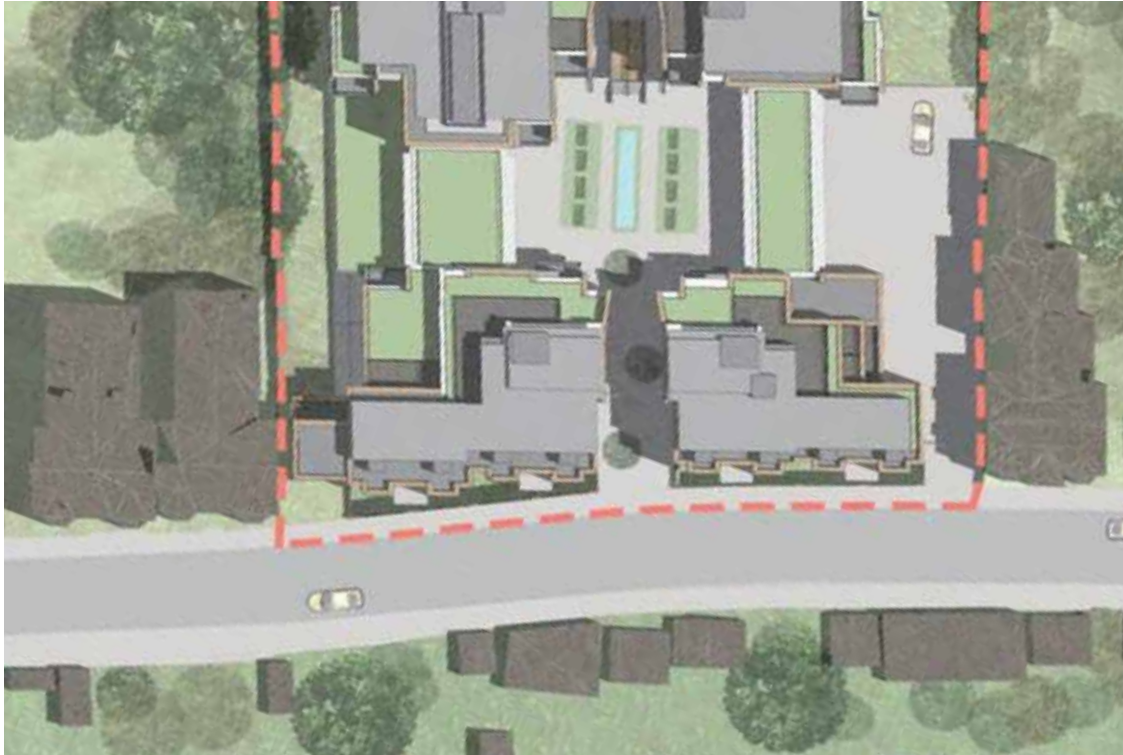
fig 3.13 Coloured plan of the proposal showing main central entry point, shared vehicle and pedestrian entry to the south, entrance courtyard and green roofs to the link blocks
