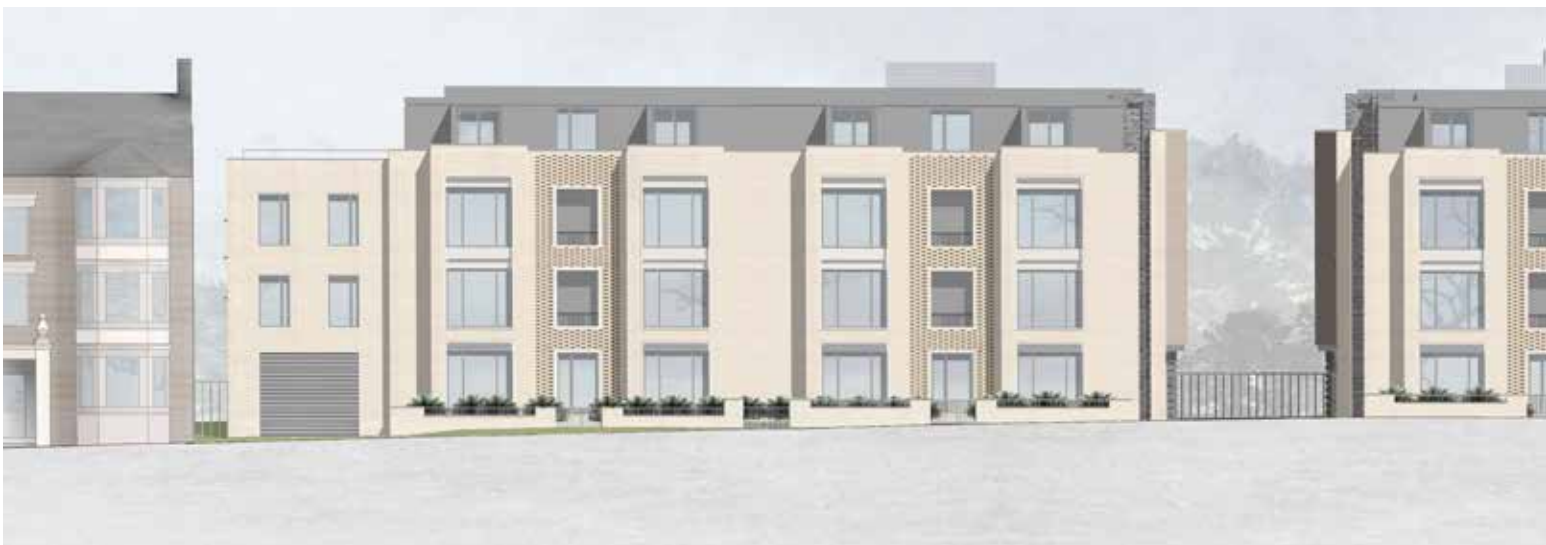
fig 3.2 Part street elevation of proposal showing size and location of windows, terraces, inset balconies and main pedestrian entrance into the development. Also the existing Chase Mansions to the north (left) of the blocks.
