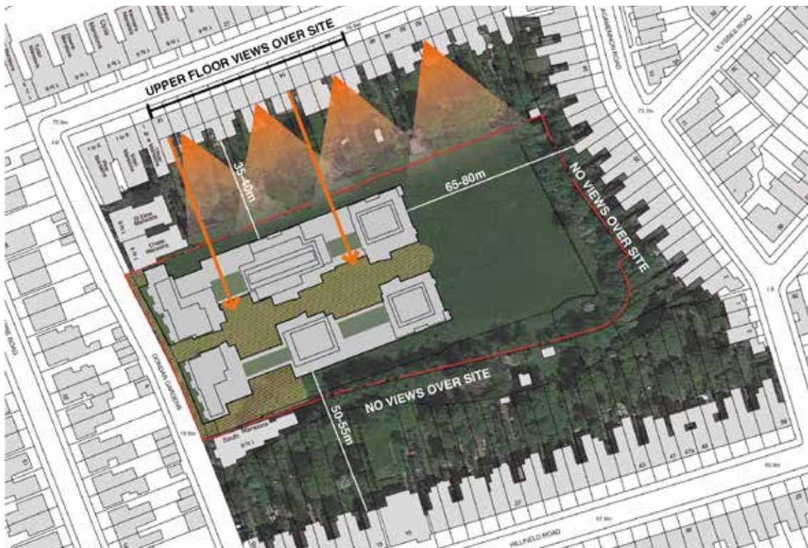
fig 3.22 See also Appendix 5.16. Plan showing limited numbers of houses with views over the site and distances from proposed new development NTS
