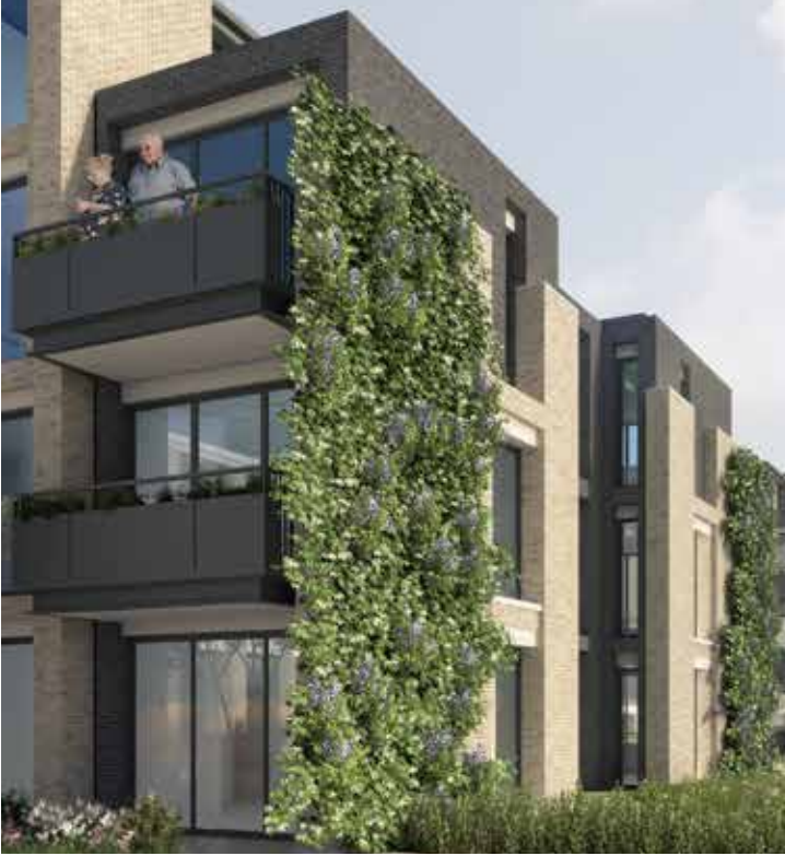
fig 3.15 View of green wall treatment to balcony edges along north and south elevations
