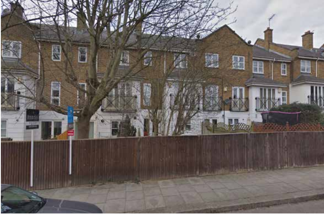
fig 3.1 More recent housing, late 20th Century, a local 'gated' development - Berridge Mews off Hillfield Rd (built 1989/90). Poor quality streetscape onto Hillfield Rd with continuous 1.8m high close boarded fence to back of pavement and no visual or physical connection into gardens or houses from the street.
