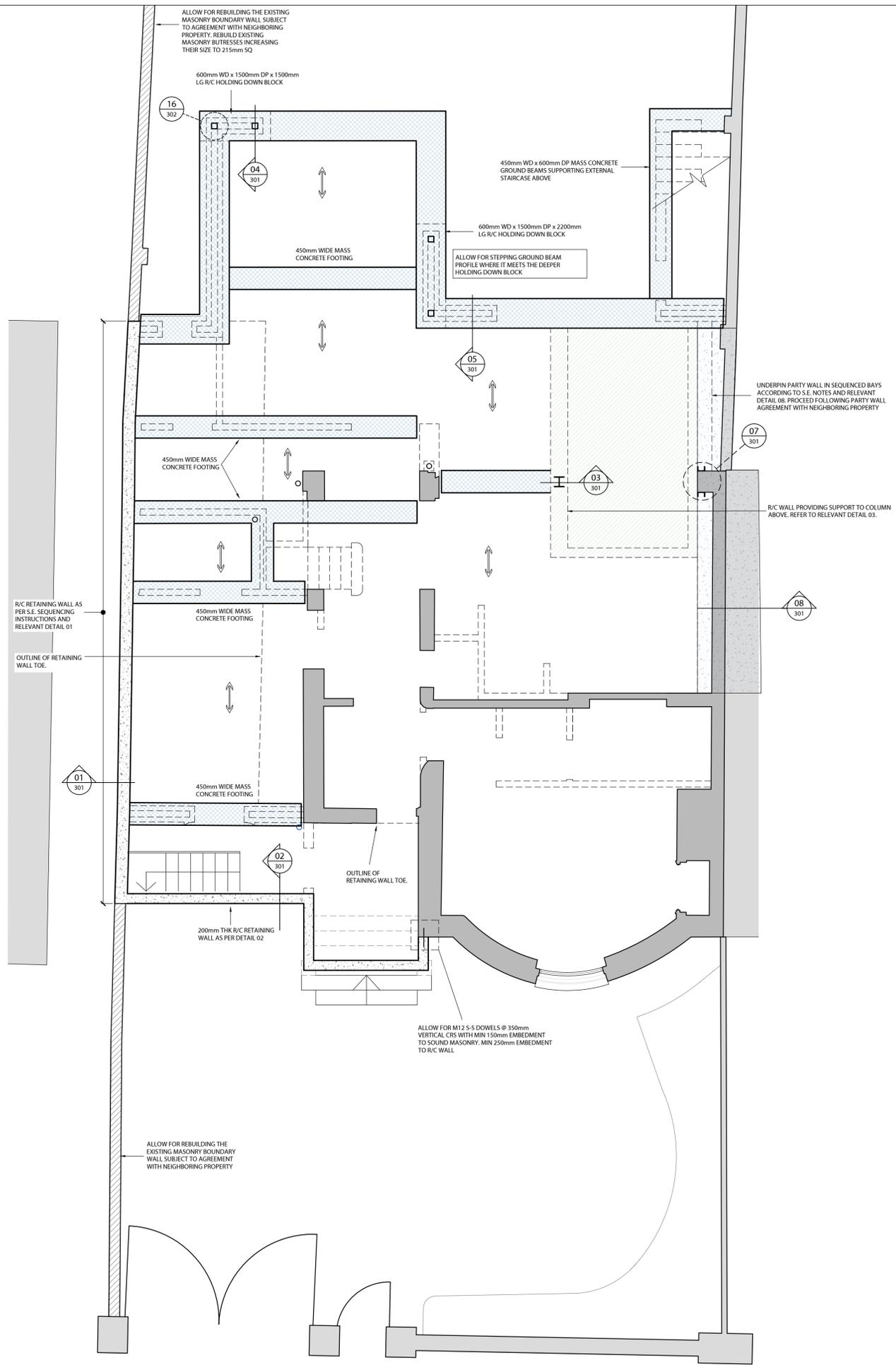
ALL PCC LINTELS HIGH SPEC NAYLOR LINTELS REF: S4 OR EQUIVALENT APPROVED UNLESS NOTED OTHERWISE. NUMBER TO SUIT FULL WIDTH OF THE WALL.
