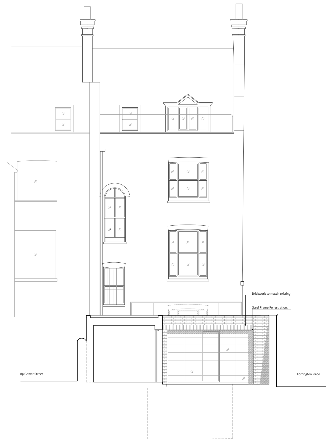
Proposed South West Elevation (Rear). 1:100.
