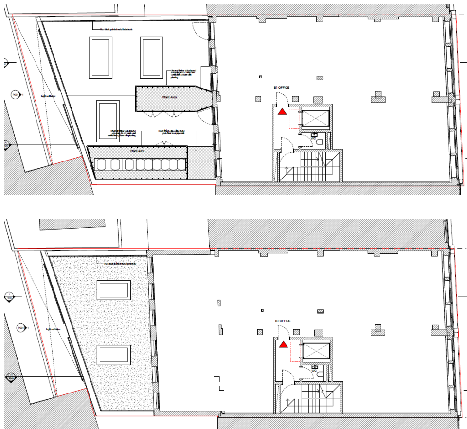
Images 6 and 7 – second floor plan with external plant (2019/2041/P) and the revised second floor plan with internal plant enclosure
