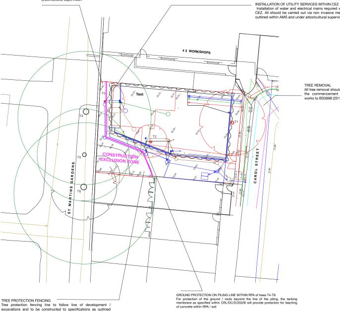
Installation of water and electrical mains required within the CEZ. All should be carried out via non invasive methods as outlined within AMS and under arboricultural supervision
