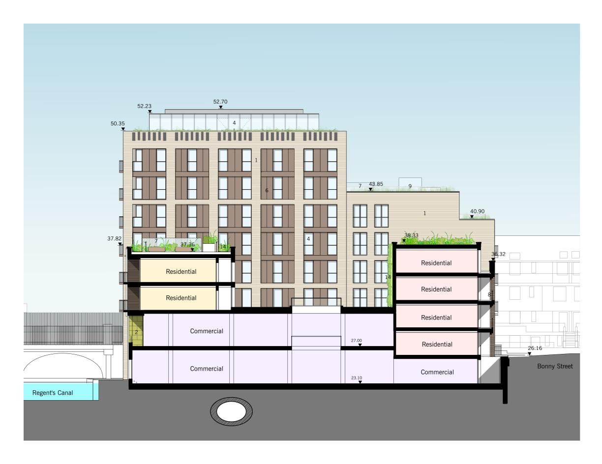
CSC5/S1NMA Approved Ref: 2017/6270/P Section DD (Block A & Block C)
