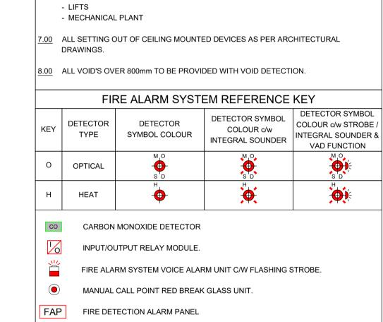
CO CEILING MOUNTED CARBON MONOXIDE DETECTOR
