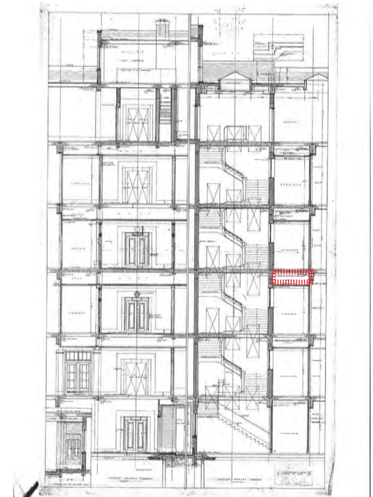
Historic E/W section through Central and West wings with existing services trench at L2 shown in red outline
